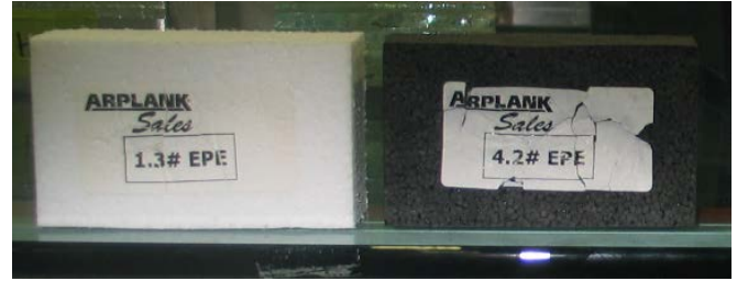
Figure 5: EPE Foam Blocks after Cold Impact Testing
