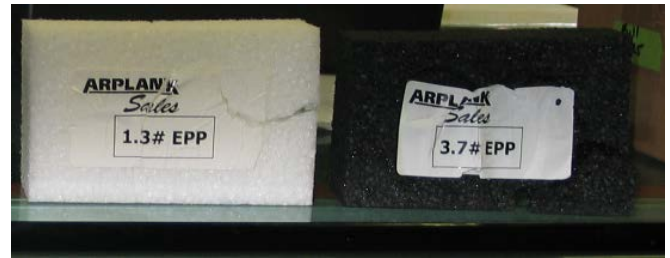
Figure 6: EPP Foam Blocks After Cold Impact Testing
